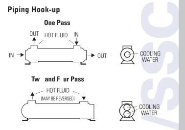
*Specific applications may have different piping arrangements. Contact factory for assistance.*
